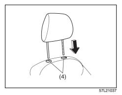
To reinstall the head restraint, insert the head restraint bars into the holes (4) and push the head restraint down.
